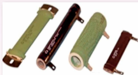
Primeri uporov, navitih z žico in cementirani
