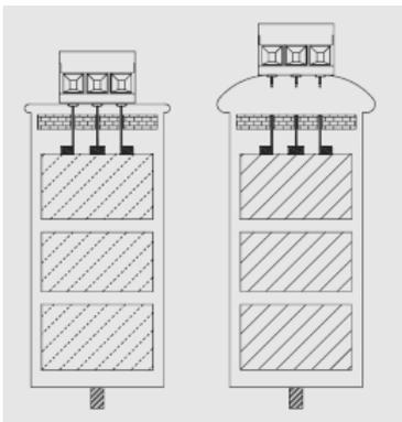
Due to extreme and inadmissible operating conditions of overvoltage, overcurrent, high harmonics or high temperature, LPC capacitors have been designed all three phases to be disconnected by an internal overpressure disconnection system, thus the terminals connection with the capacitive element is interrupted.
